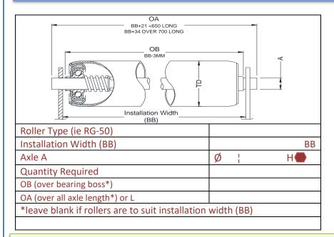
Bearing housing: steel swaged
