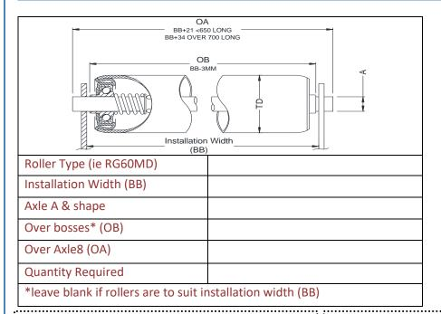
Bearing housing: steel swaged
