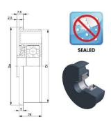
PRP series are general purpose plastic rollers with sealed plastic housed SS precision bearing (pop metric) for manual/under belt applications
